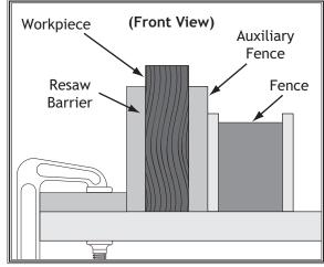
**Figure 61.** Example illustration of a resaw setup.
